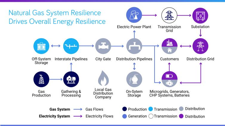
Natural gas infrastructure is critical to supporting gas-powered electric generation systems – this is central to ensuring resiliency of the overall energy system.
